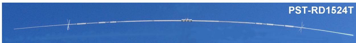
Install antenna on your mast, make sure to have almost 5-6meters or 15-20 ft over the roof or ground and if installed over an HF yagi antenna, make sure to have dipole in line with yagi's boom spacing them almost 2m or 8 ft. Antenna will have the best performance if installed almost a  $\frac{1}{4}$  wave of the lower frequency band, over the ground.
